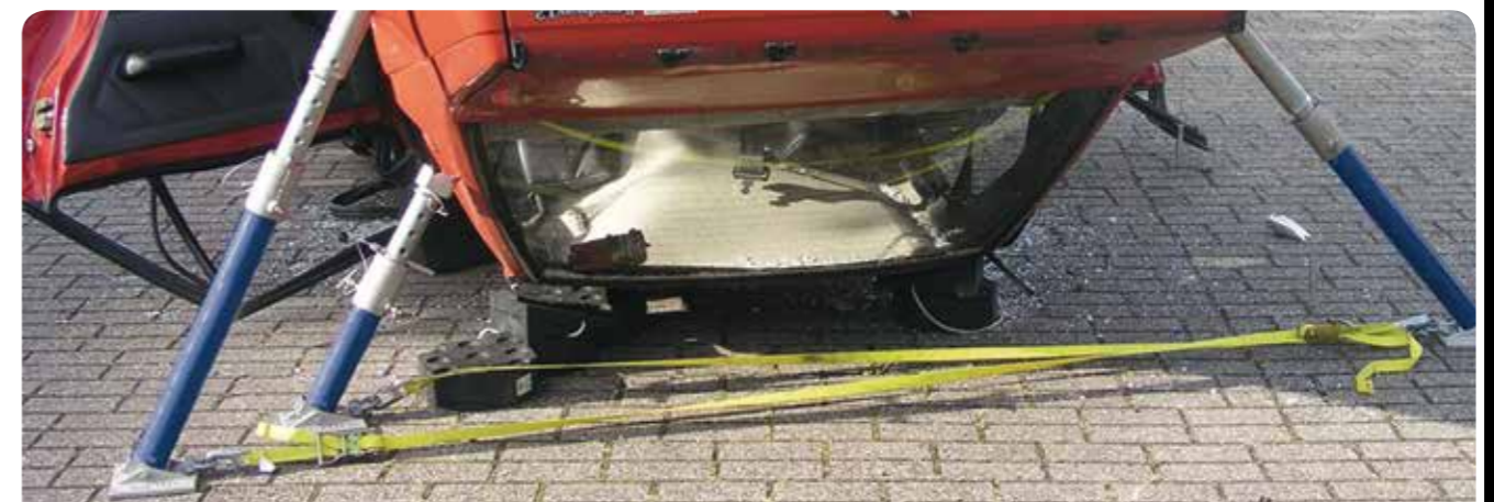
Vehicle stabilisation with ART-Lite strut.
