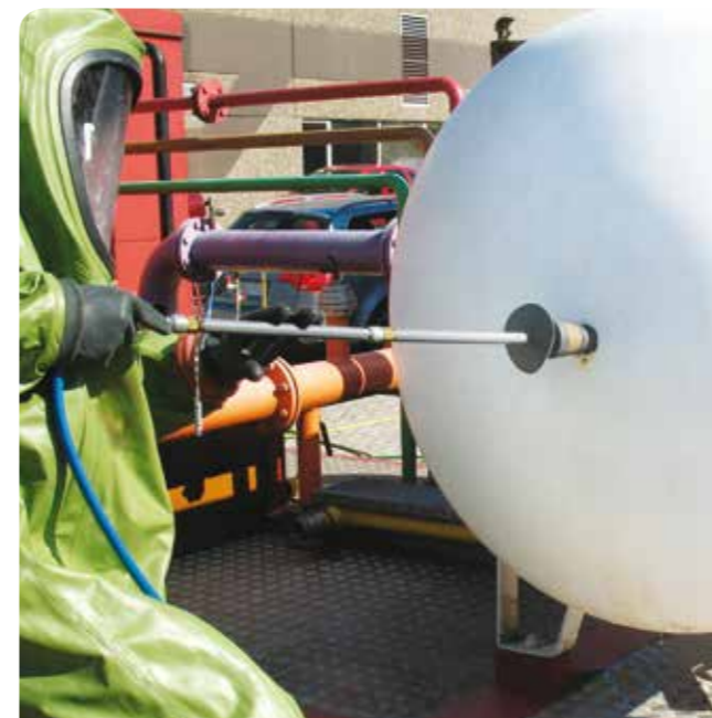
Seal leaks from a safe distance.
