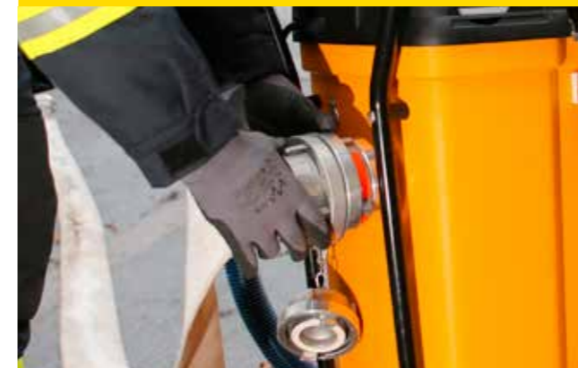
Connection for fire-service hose
