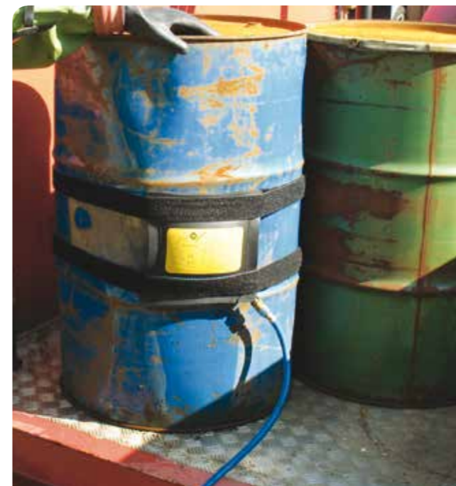
Sealing bags stop drum leaks.
