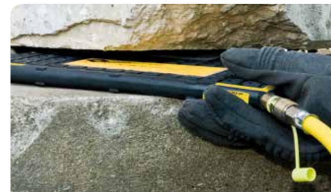
Uniform low insertion height of 2.5 cm (0.98 inch) for all bag sizes.
